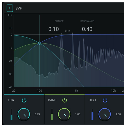
SVF response display — LOW, BAND, and HIGH branches share Cutoff and Resonance
