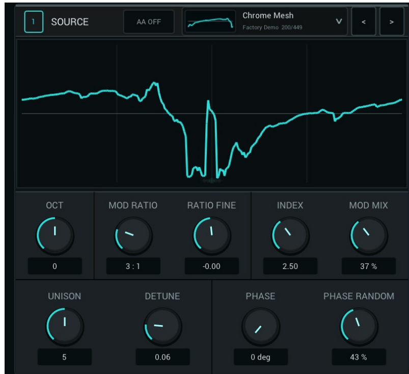
Source — waveform, anti-alias mode, FM controls, unison, and phase
