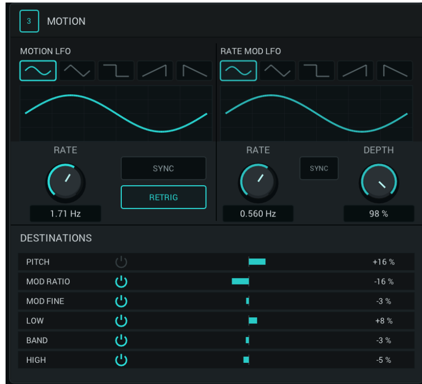
Motion — main LFO, Rate Mod LFO, and six signed destinations
